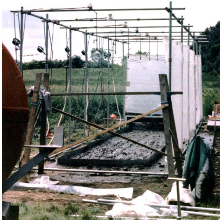
Figure 3.6. Rainfall simulator for an outdoor runoff plot experiment.
