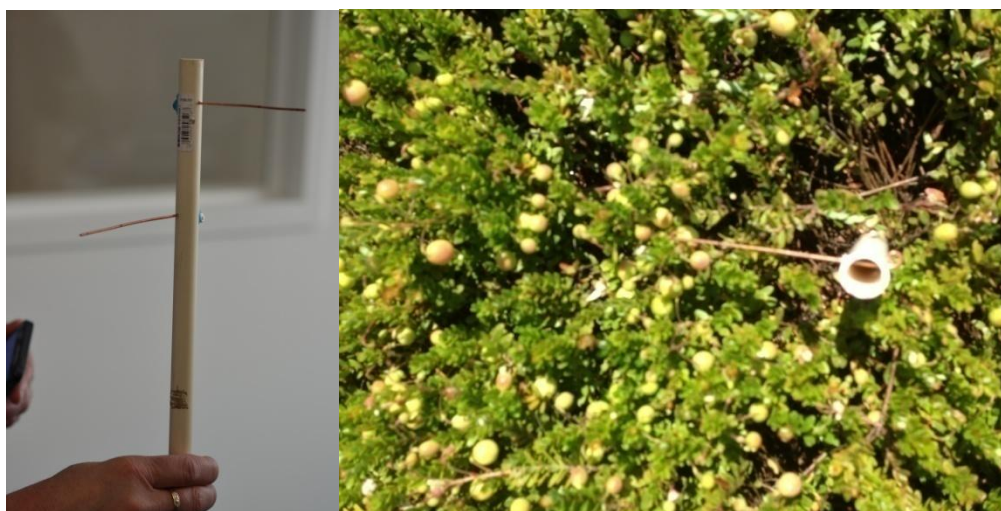
Fig. 4. Horizontal copper sticks fixed to a PVC tube (left) and top view of targets set up in the field (right).
