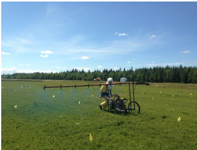
Fig. 1. Spraying with boom set to 1.2 m (August 6 2013).
