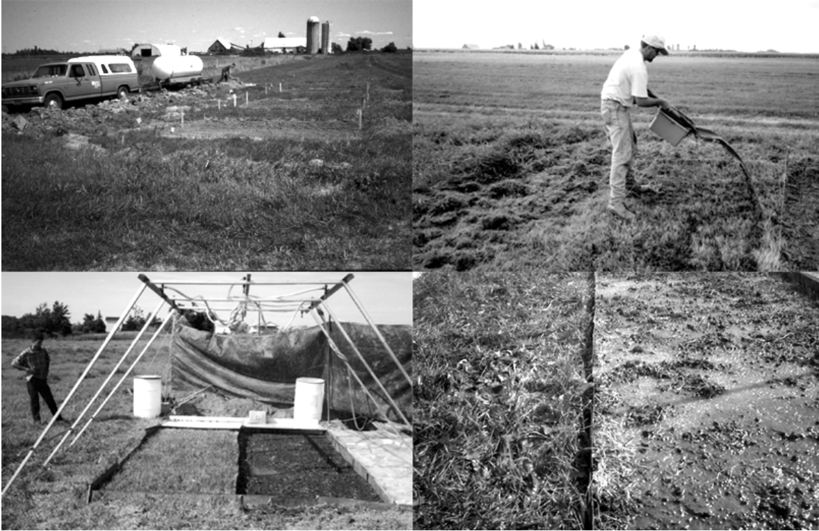
Figure 1 : Experimental set-up for simulated rainfall runoff plot study on benchmark soils of Castors brook watershed.
