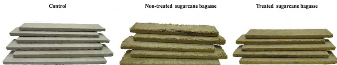
Fig. 4 – Prismatic specimens (250 mm × 50 mm × 10 mm) of the composites fabricated for the mechanical tests.
