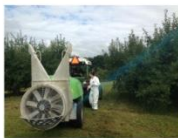
Figure 3. Calibration of conventional orchard sprayer
