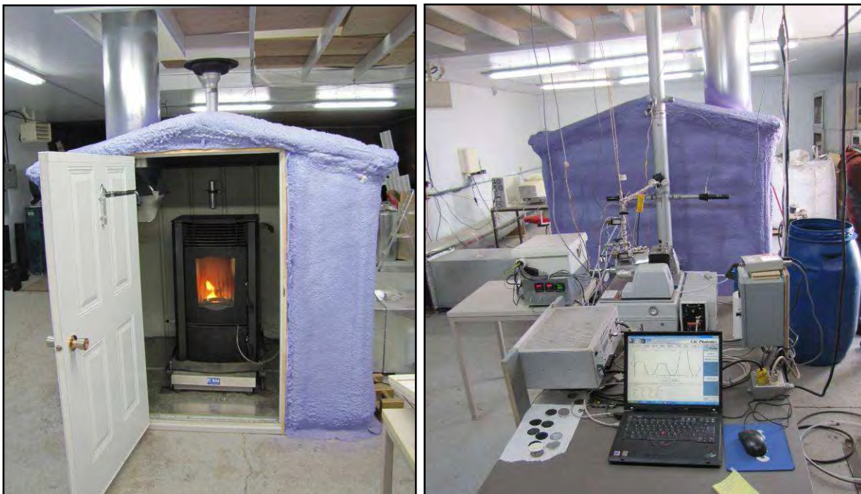
Fig. 2. Biomass combustion test setup, front view (left) and rear view (right).
