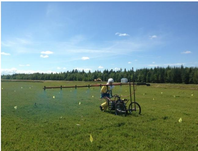
**Fig. 1.** Spraying with boom set to 1.2 m (August 6, 2013).
