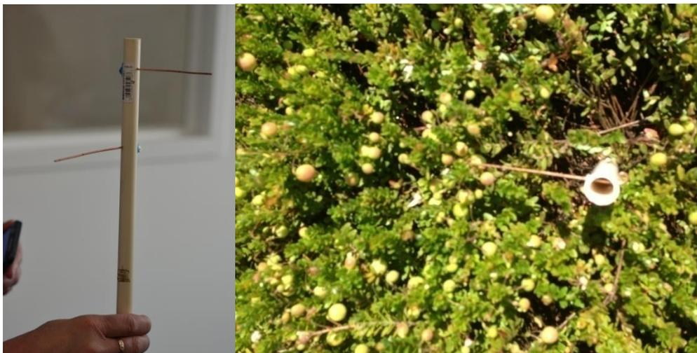
**Fig. 4.** Horizontal copper sticks fixed to a PVC tube (left) and top view of targets set up in the field (right).
