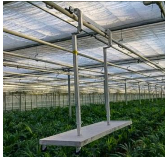
Source : De Velle – Monorail carrier with platform
